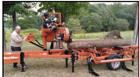
Ross Clair, Northeast Wood-Mizer dealer from Maine demonstrates how to properly saw a log with the LT 40 mill at the Urban Forestry Center.
